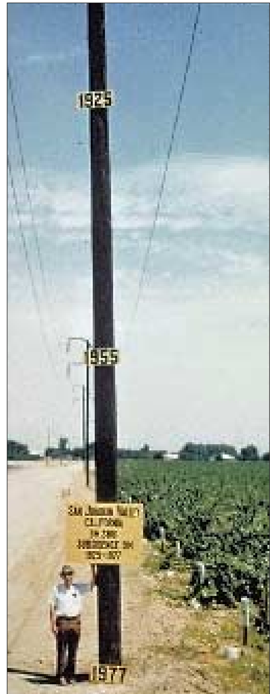
Figure 5. A dramatic example of subsidence in California showing the drop in land elevation from 1925 to 1977 ( http://water.usgs.gov/pubs/circ/circ1182/pdf/06SanJoaquinValley.pdf ).
