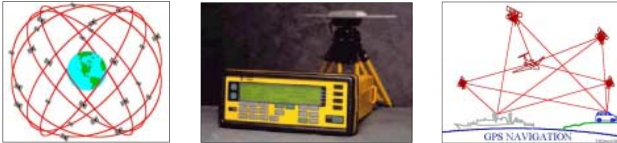
Figure 4. The global positioning system (GPS). Left image: Composed of 28 satellites orbiting the earth at 20,200 km ( http://www.colorado.Edu/geography/gcraft/contents.html ). Center image: A Trimble GPS receiver and antenna ( http://www.trimble.com/products/pdf/geosurvey.pdf ). Right image: GPS navigation is independent of physical landmarks ( http://www.colorado.Edu/geography/gcraft/contents.html ).
