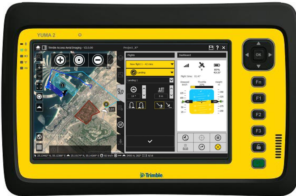
Trimble Yuma 2 tablet running the Trimble Access Aerial Imaging software
