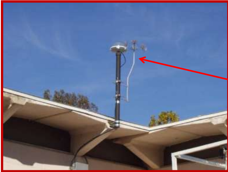
Problem tribrach "feet" cannot be locked height can be changed
