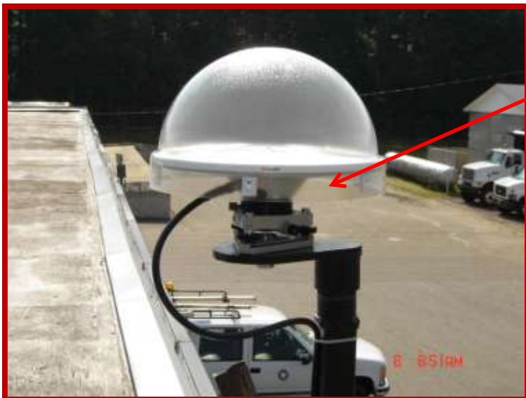
Problem tribrach "feet" cannot be locked height can be changed
